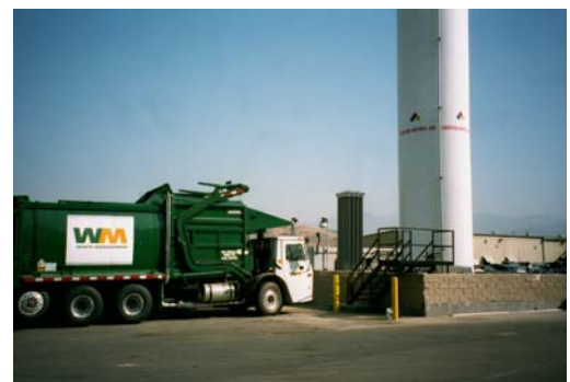
Waste Management LNG Refuse Truck at Fueling Station in Corona, CA
