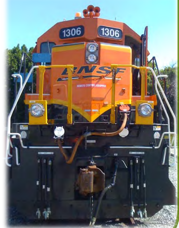
Generator set switch locomotives significantly reduce NOx & PM
